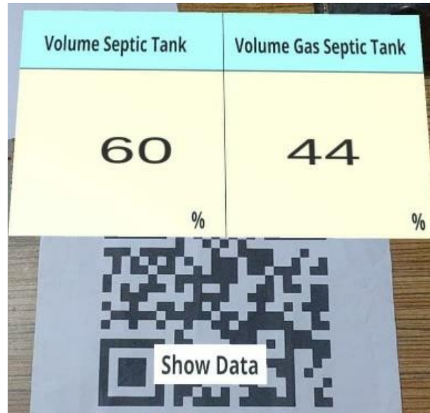
Figure 5. Augmented reality application using Unity with the Vuforia SDK
